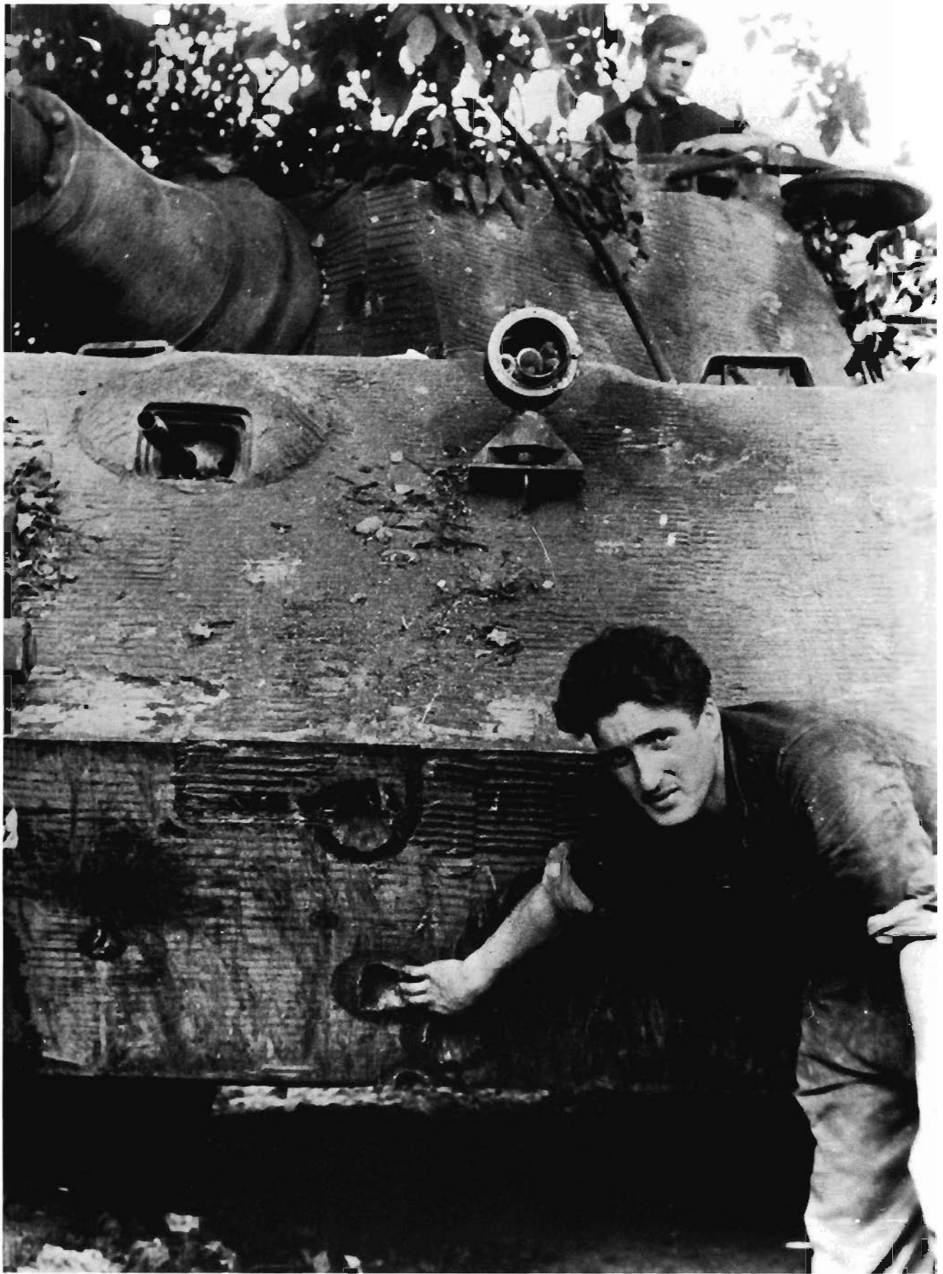
The caption on this print states 'Invasionsfront', which would seem to prove the existence of at least one Henschel-turreted Königstiger in Normandy. The frontal armour is 100mm thick —
