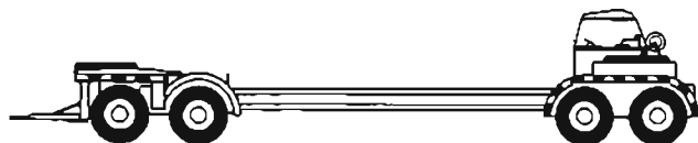
Tieladeanhangter, SdAk 116 (22-ton tank transporter trailer)
