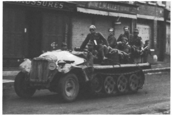
An m.Zgkw 8t. (SdKfz 7) eight-tonne medium prime-mover followed by the one-tonne le.Zgkw 1t (SdKfz 10). (Bundesarchiv)
