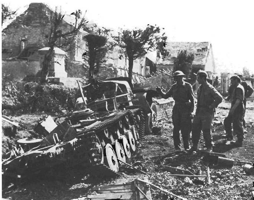
Although there is no positive proof that this Maultier belonged to the Panzer Lehr Regiment, it makes a nice comparison in Monts-en-Bessin, the village where Generalleutnant Fritz Bayerlein, divisional commander, had his HQ. The Maultier was a 4½-tonne Mercedes-Benz truck with the rear axle assembly replaced by tracked suspension and used as a cargo carrier. (IWM)
