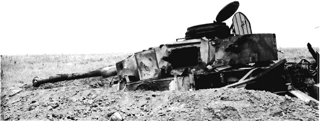
Nearby, another Mk IV from the II. Abteilung also received a direct hit on its turret. This shell appears to have struck from the opposite side, smashing the 30mm armour beside the hatch and blowing off the skirt. (IWM)
