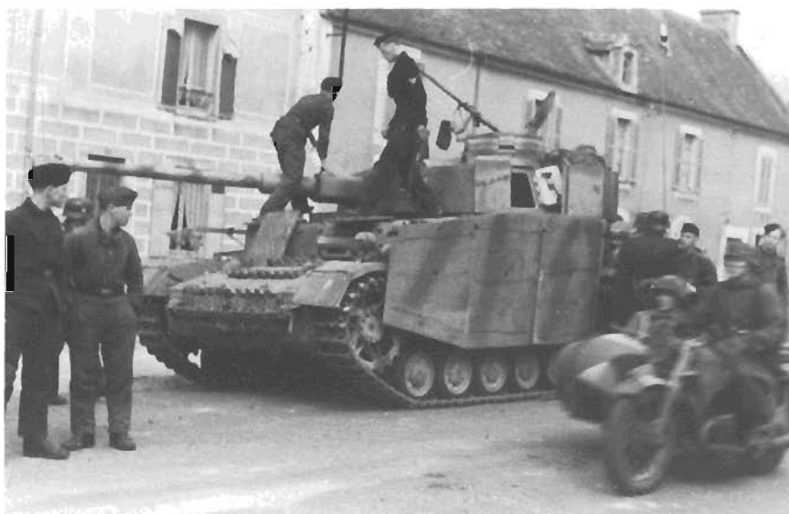
Tankers from an army panzer unit with their Ausf H. The schürzen afforded a measure of protection to the sides of the body and turret. Constructed of 5mm mild steel boiler plate, these skirts would prematurely explode a projectile several inches in front of the armour. The wires have been added for attaching camouflage foliage. The turret machine gun is the 7.92mm MG34. (Bundesarchiv)
