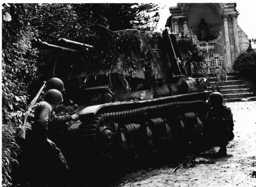
Renault R-35 chassis with a Czechoslovakian 47mm anti-tank gun in German service . . . or rather, late of the German army. (US Army)
