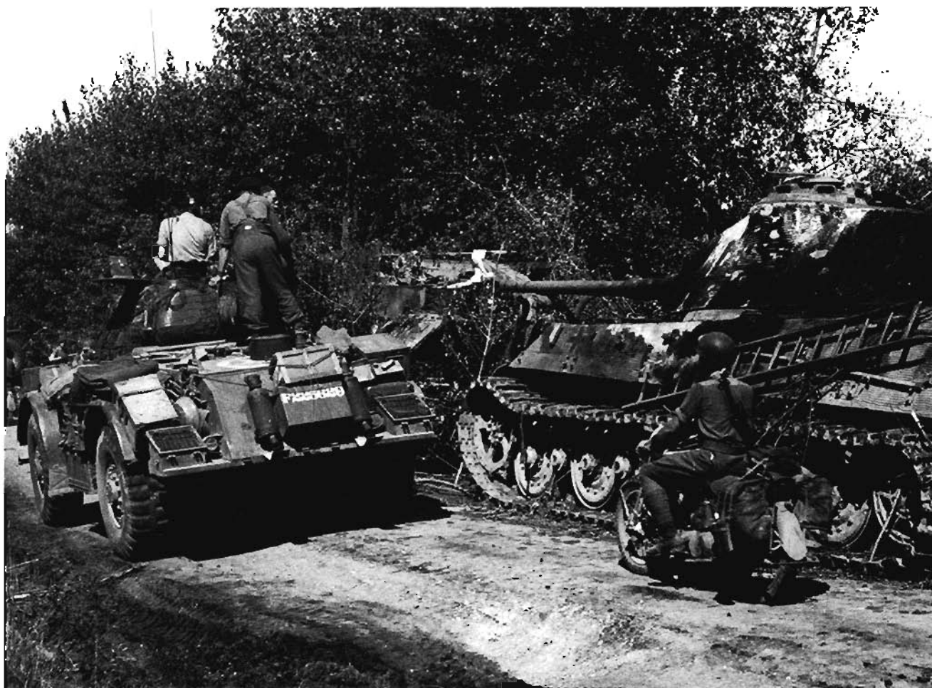
Very interesting photo from Canadian archives showing a King Tiger abandoned while being towed by a Bergepanther — one of only two such recovery vehicles on the strength of the 1. Kompanie of schwere Panzer Abteilung 503. The picture was
